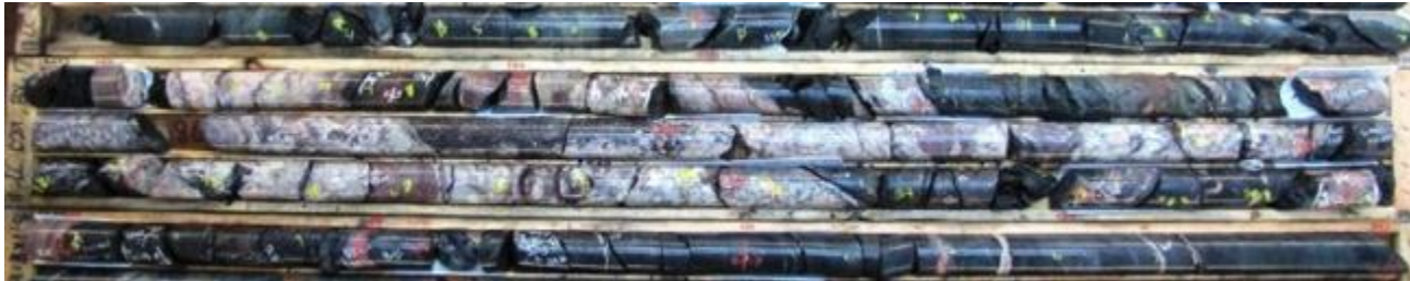
11-LC-029 Main Zone HW 84.4m to 84.9m = 0.25% U 3 O 8 / 0.5m (0.5mTW) & Main Zone FW 87.2m to 89.0m = 0.08% U 3 O 8 / 1.8m (1.6mTW)
