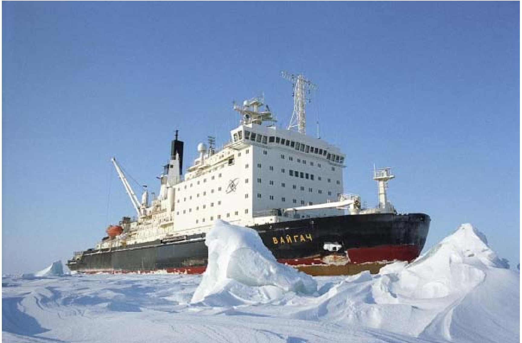
Taymyr class icebreaker powered by two KLT-40 nuclear reactors
